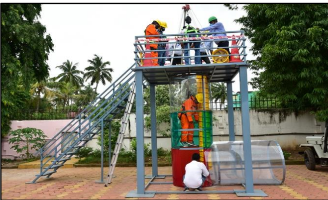
Figure 6: Entry procedure of professionals into the sewer maintenance hole
