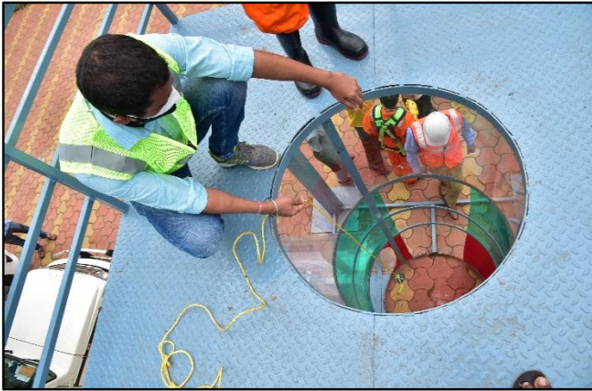
Figure 4: Gas testing inside the maintenance hole
